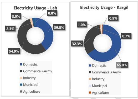
Figure 8: Electricity Consumption in Leh and Kargil
